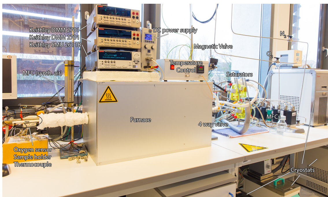
Figure 6.12: Photography of the experimental setup for ECR measurements at RWTH Aachen University, Institute of Physical Chemistry, High Temperature Laboratory 2400|131.
